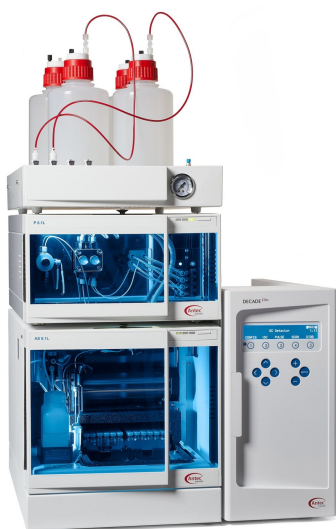
Figure 1. ALEXYS Carbohydrate Analyzer consisting of the ET 210 eluent tray (for \text{N}_2 blanketing), a P 6.1L quaternary LPG pump, AS 6.1L autosampler and the DECADE Elite electrochemical detector.
